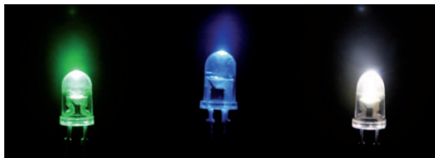
Figure 1. Green- and blue-emitting ( \text{Ga}_{1-x}\text{In}_x )N LEDs (left and center) and a blue LED coated with the yellow illuminant Ce-YAG ( \text{Y}_3\text{Al}_5\text{O}_{12}:\text{Ce}^{3+} , right).
